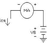
II.5. Now disconnect the test circuit, and connect the current source in place of the fixed emitter resistor in the differential amplifier (no Si diode is needed now). Verify that the Q point of the diff amp is essentially the same with the current source as it was with the fixed emitter resistor; if it isn't, slightly adjust the  $20K\Omega$  trim pot to make it the same.
