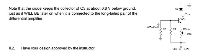
Then build the current source, but **do not connect it** to the Diff Amp. Use a 20K pot for  $R_E$  and adjust it to make the collector current of the current source to be the same as the long-tailed pair current (measured in I.2.), but DON'T connect it to the diff amp yet.
